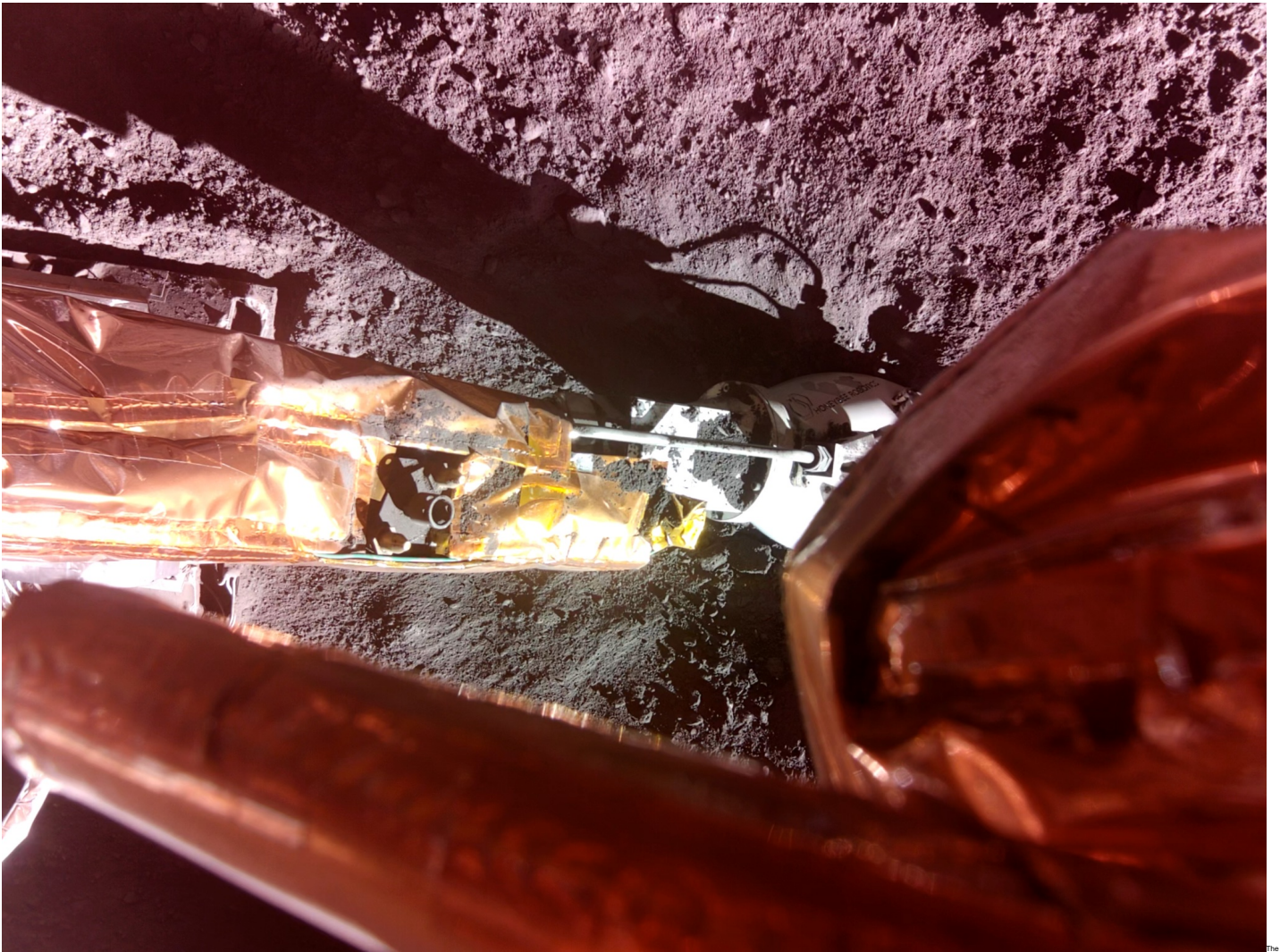
Lunar PlanetVac instrument, developed by Honeybee Robotics, was deployed to the lunar surface and is shown at the end of Blue Ghost's surface access arm. Credit: Firefly Aerospace
