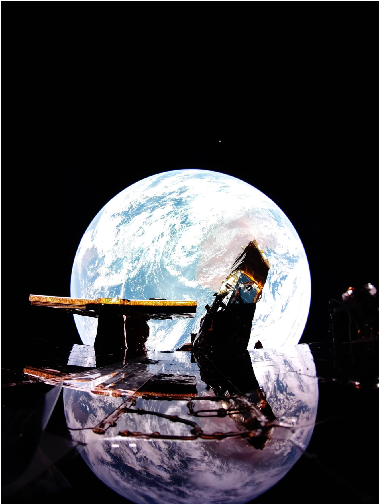
captures image of Earth reflecting off the solar panel with the Moon on the horizon above Earth. Firefly's X-band antenna and NASA's LEXI payload are also shown on the top deck of the lander. Credit: Firefly Aerospace
