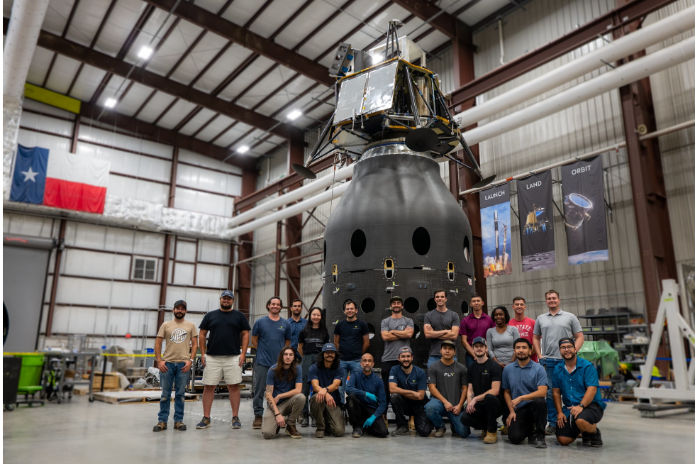
Blue Ghost Mission 2 structure qualification model fully stacked with Blue Ghost lander, Elytra Dark vehicle, and dual payload attached fitting at Firefly's Rocket Ranch in October 2025.
